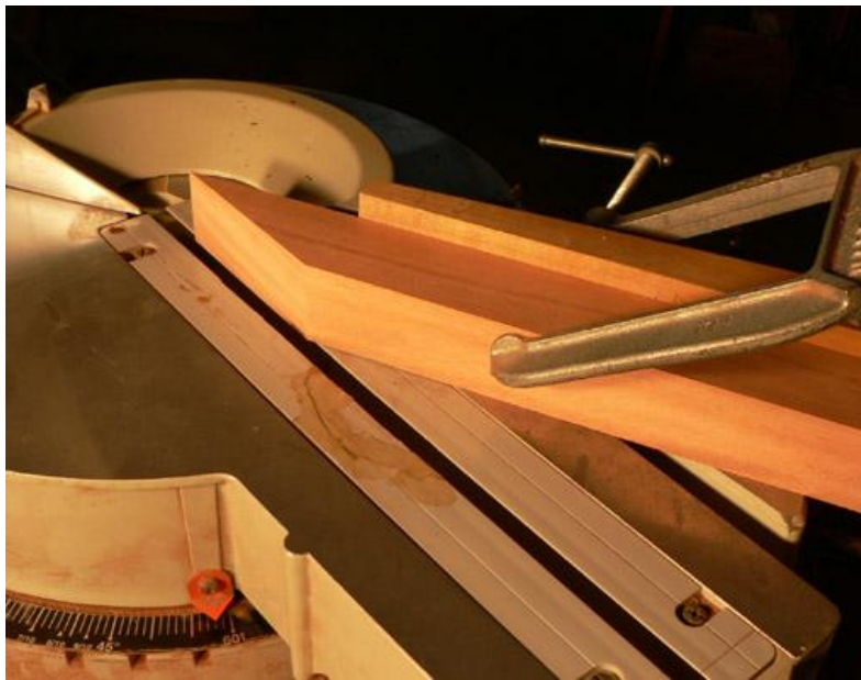
Photo 2. Cutting a 27° mitre on a sliding mitre saw, using a 5° wedge clamped between the workpiece and the fence. You must ensure that the blade will clear the clamp before making the cut.
