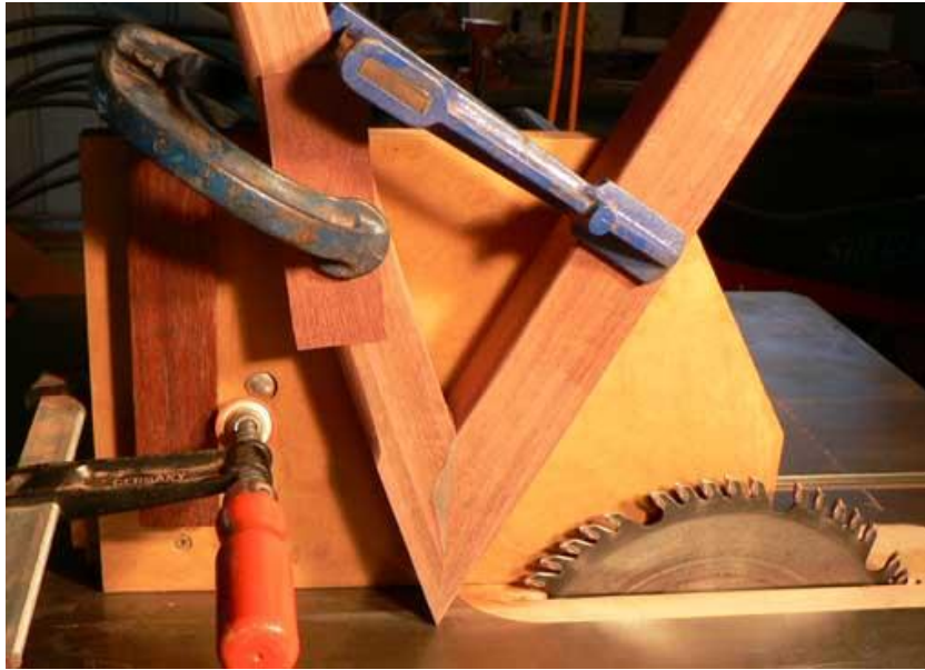
Photo 5. Cutting the kerfs for the mitre keys.
