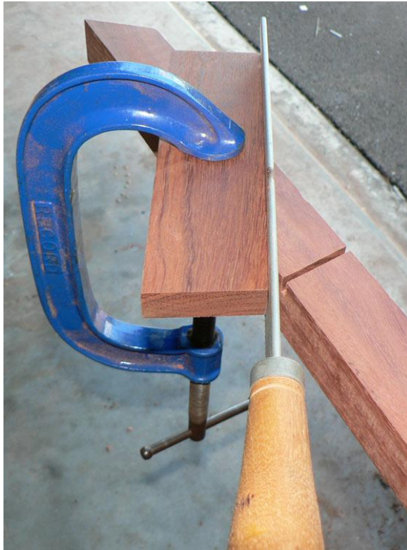
Photo 7. Cutting the housing on a back stile.
