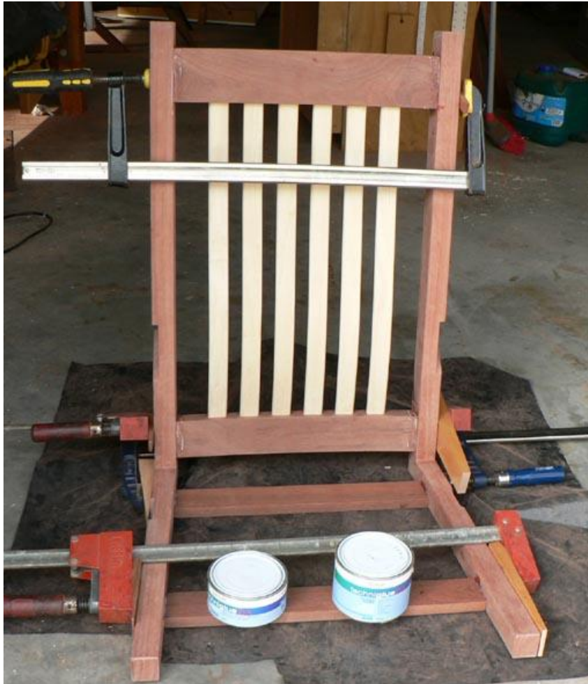
Photo 8. Glueing up the seat/back assembly.
