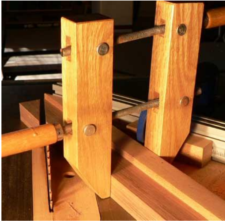
Photo 3. Cutting a mitre on the table saw with a jig clamped to a mitre gauge.
